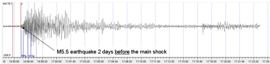
Figure 1: Before the main shock. A M5.5 earthquake recorded at station ERM, located 700km north of the epicenter. The seismogram does not display variation of low frequency.
