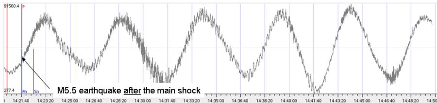
Figure 2: After the main shock. An earthquake of similar magnitude, recorded at the same station. The seismogram shows important low frequency component.
